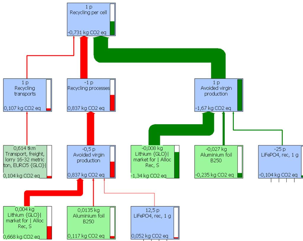
Figure 4 Model of recycling of 149.7 g lithium cell – avoided climate impact
