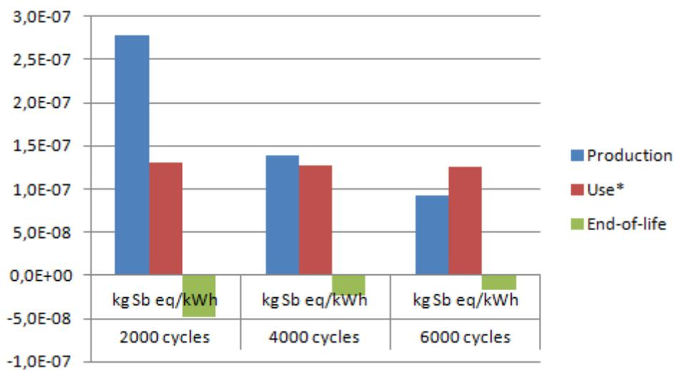
Figure 12 Abiotic depletion, kg Sb-eq per delivered kWh (2000, 4000 and 6000 cycles at  $\eta=0.9$ ). \*Use phase impacts cover only battery related losses.
