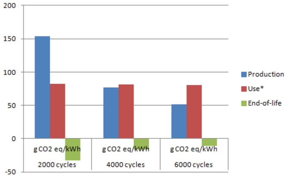
Figure 9 Climate impact per delivered kWh for TriLi 5 Ah cell (at 2000, 4000 and 6000 cycles at  $\eta=0.9$ ). \*Use phase impacts cover only battery related losses.
