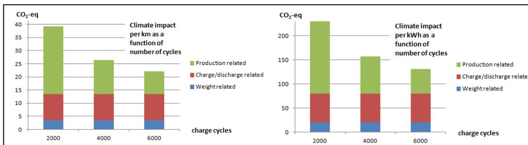
Figure 5 Climate impact CO<sub>2</sub>-eq per km and per kWh as a function of number of cycles
