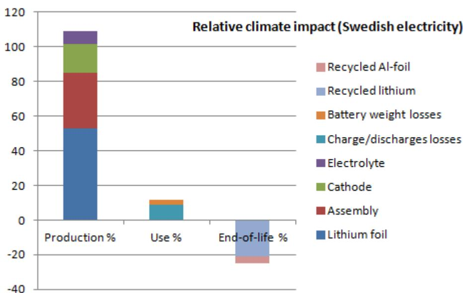
Figure 15 Relative climate impact (18.4 kWh, 4000 cycles,  $\eta=0.9$ )
