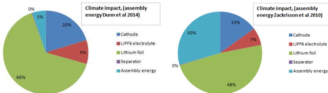
Figure 18 Relative climate impact of production of 5 Ah cell with different assembly energy approximations
