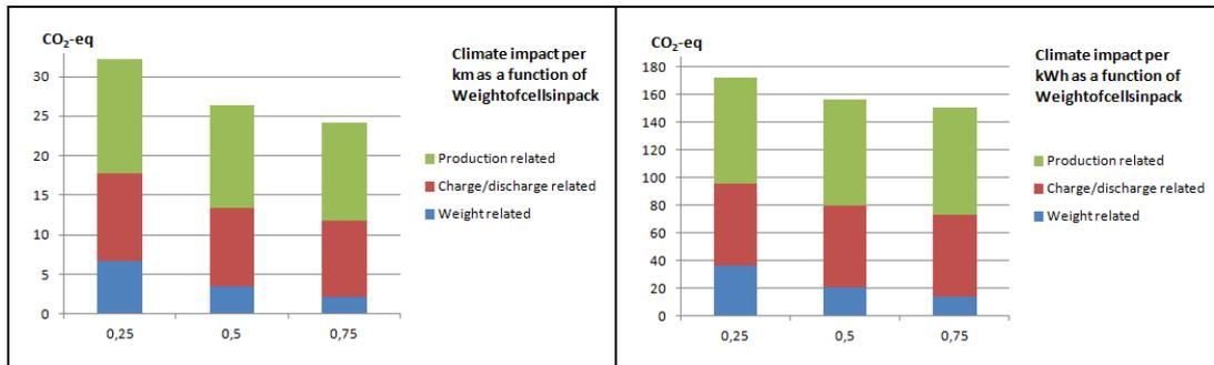
Figure 7 Climate impact CO<sub>2</sub>-eq per km and kWh as a function of the cell weight related to battery weight
