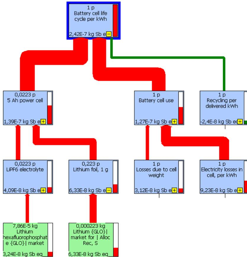
Figure 11 Abiotic depletion, kg Sb-eq per delivered kWh for The 149.7 g 5 Ah cell (4000 cycles,  $\eta=0.9$ , European electricity)
