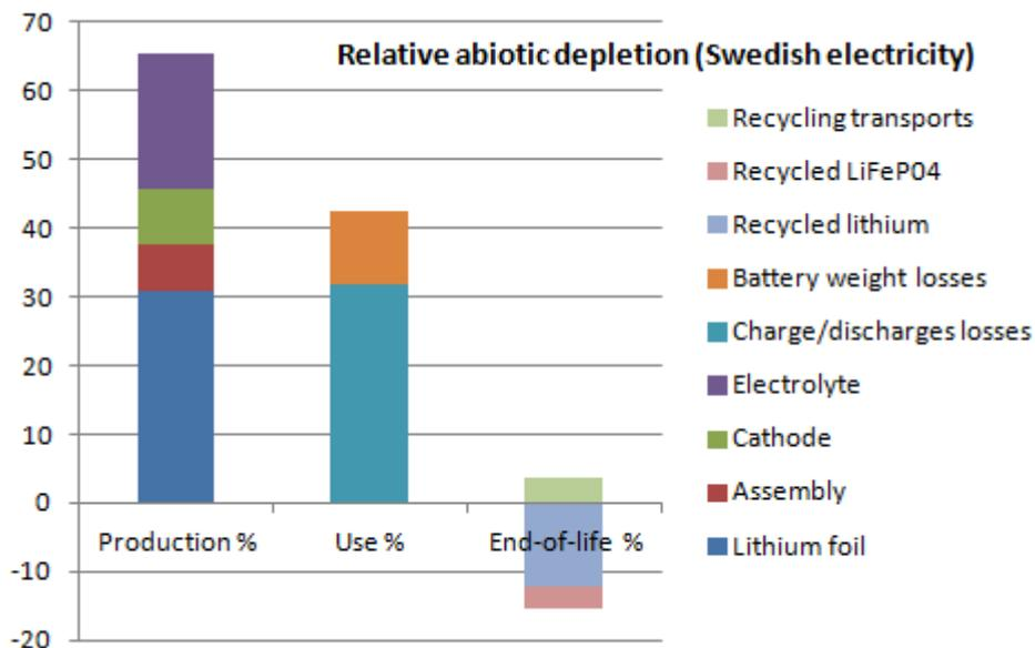
Figure 16 Relative abiotic depletion (18.4 kWh, 4000 cycles,  $\eta=0.9$ )
