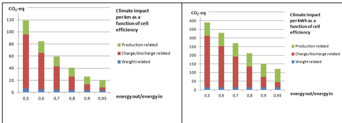
Figure 6 Climate impact CO<sub>2</sub>-eq per km and kWh as a function of cell efficiency
