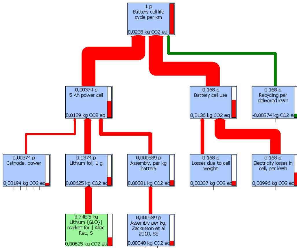
Figure 8 Climate impact per vehicle km for 149.7 g 5 Ah cell (10.8 kWh battery, European electricity)
