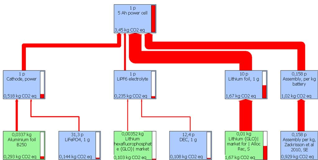
Figure 3 Production of 149.7 g lithium cell – climate impact
