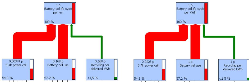
Figure 10 Climate impact per delivered kWh (right) and per vehicle km (left) for 149.7 g 5 Ah cell
