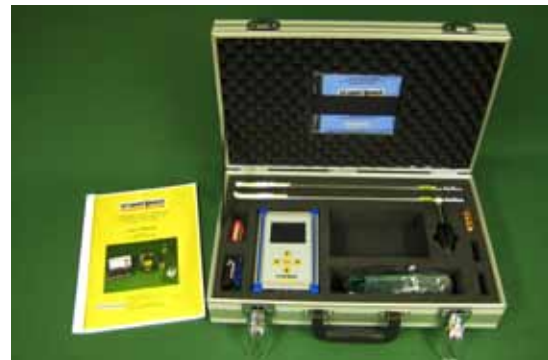
The data acquisition unit with accessories, the test probe with handle, a CD with the computer software and the manual are all contained in a carrying case.
