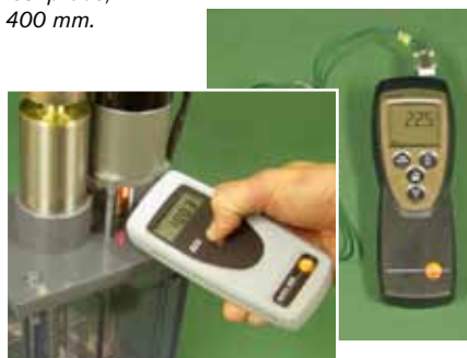
Optical tachometer with reflecting tape.
