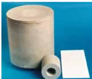
Component made by direct casting.
