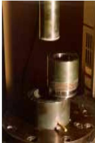
*Filter pressing offers an opportunity of simulating pressure casting on a small scale, evaluating mould materials and characterising the casting behaviour of slips.*
