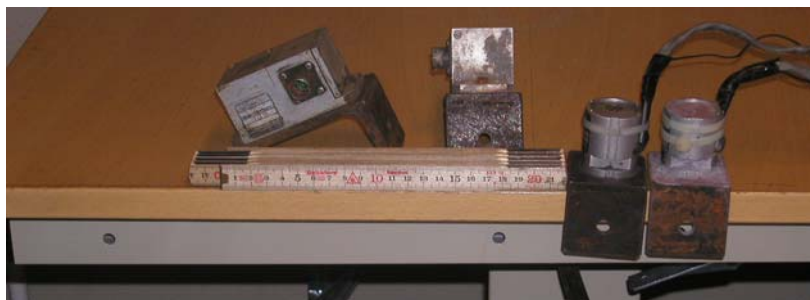
Inclinometers fixed to mounting brackets for easy handling
