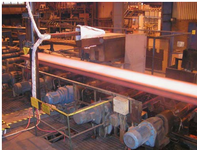
Laser sensor measuring slab position
