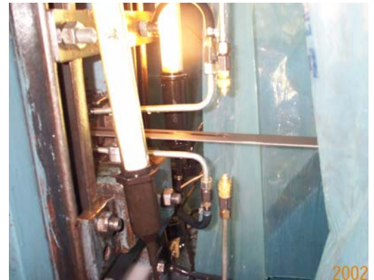
Nozzle set-up for strip and for roll gap lubrication
