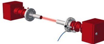
Cross duct measurement set-up with transmitter and receiver.
