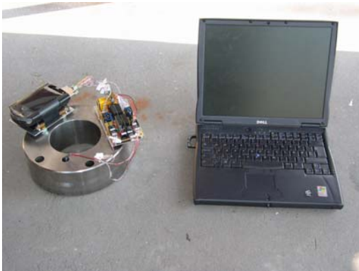
Work roll with transducer mounted inside. Amplifier and Pocket PC mounted outside the roll. Radio link connection to the Laptop PC
