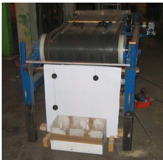
Example of measurement situation at the end of a conveyor with material falling over. The image processing system counts the size and amount of pieces falling down for further analysis.
