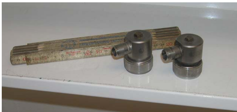
Accelerometers mounted by magnetic force
