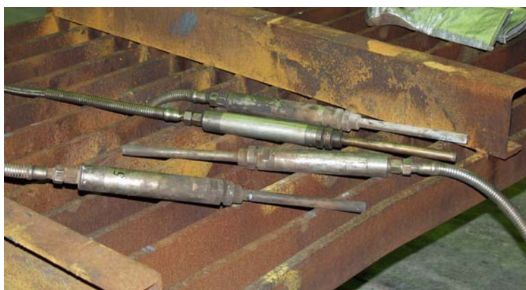
Four pyrometers developed for temperature measurements in continuous casting machines
