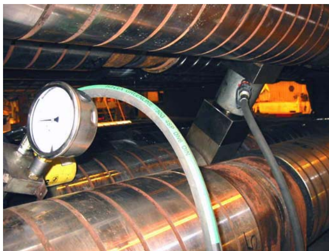
Roller apron with hydraulic jacket set-up for calibration of strain gauges
